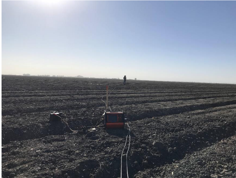
Figure 4 The WalkTEM instrument. A Ramboll staff is taking the GPS coordinates of the loop center.
