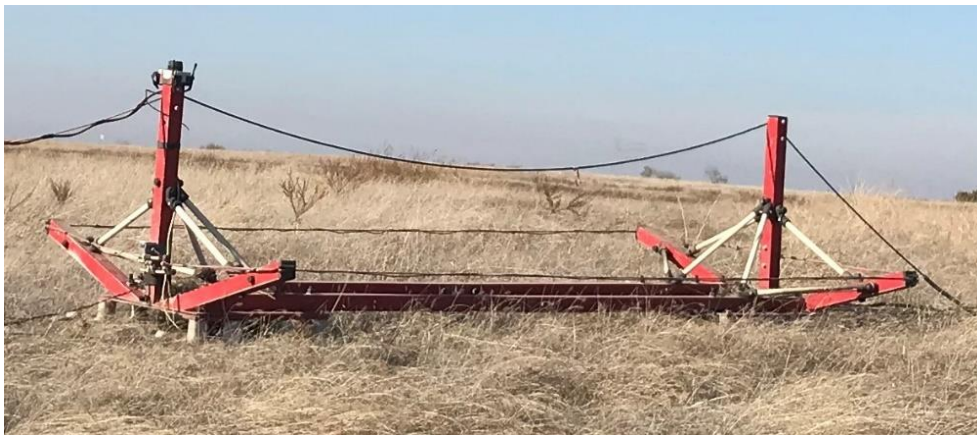
Figure 3 The tTEM transmitter sled setup at Wohle's Field.
