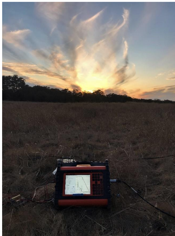
Figure 2 The WalkTEM system in operation at Santo's Field I.
